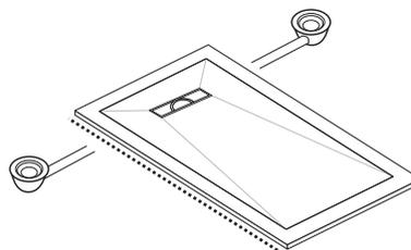
The waste outlet can be fitted left and right making installation easier. When plumbed to the right, flow will be reduced to approx. 20-25lpm.
